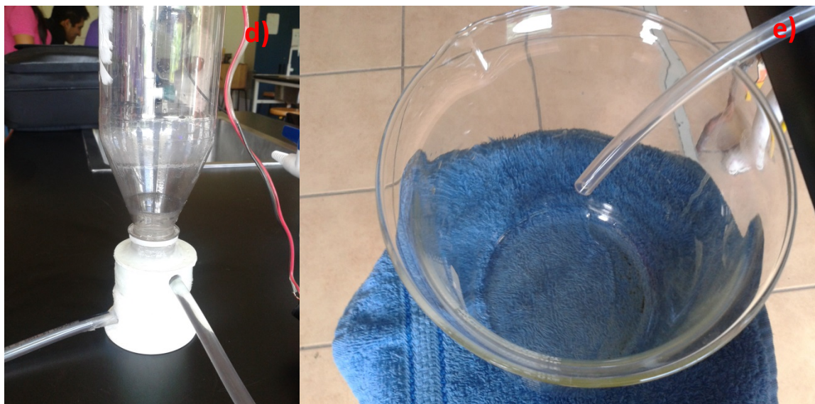
Figure 2. Process of treatment of the wastewater of the river Taxco. d) Oxygenation, and e) Container collector.
